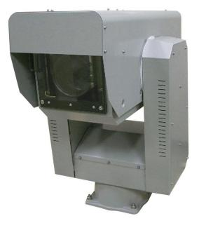
Combination of super-high sensitivity camera and 35x large magnification lens, enables long-distance color shooting in darkness.
